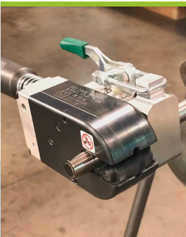
Figure 11: Remote pipe-cutting equipment
